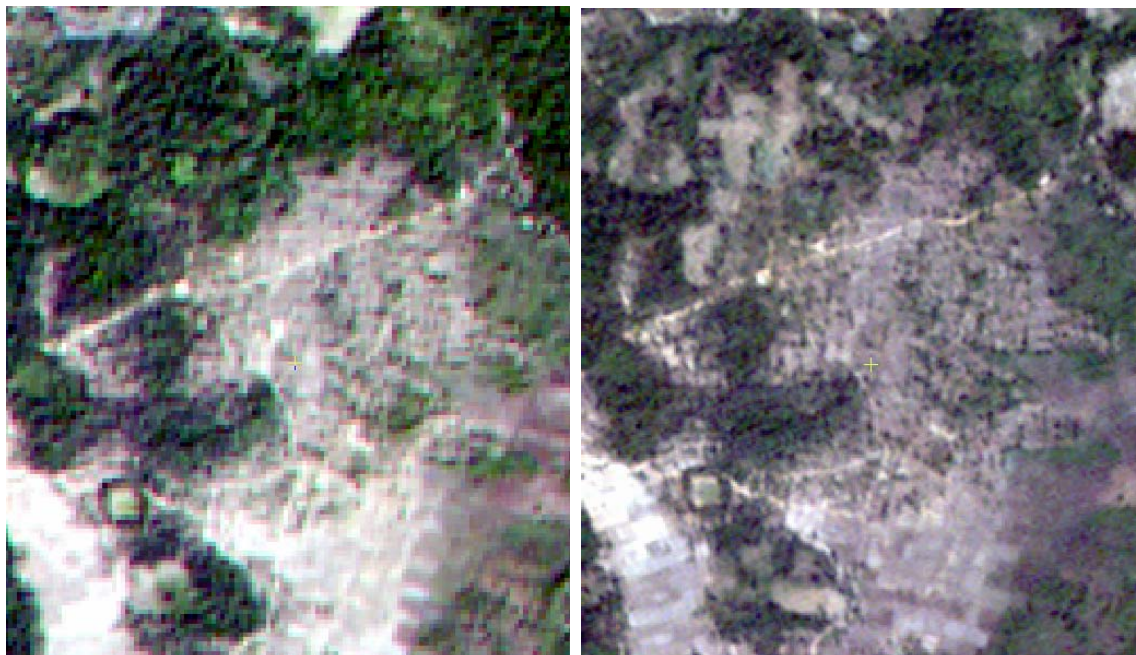
Figure 9: 10m ALOS/AVNIR-2 (Left) and 5m RapidEye (Right). Note that it is easier to discern areas of low canopy woodland in the image on the right.
